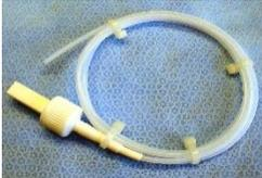
6. Place the Helix test device close the bottom of the sterilizer and sterilize it together with the load.
