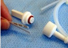
3. Insert the folded indicator strip with the closed end first in the cap of the Helix test device.
